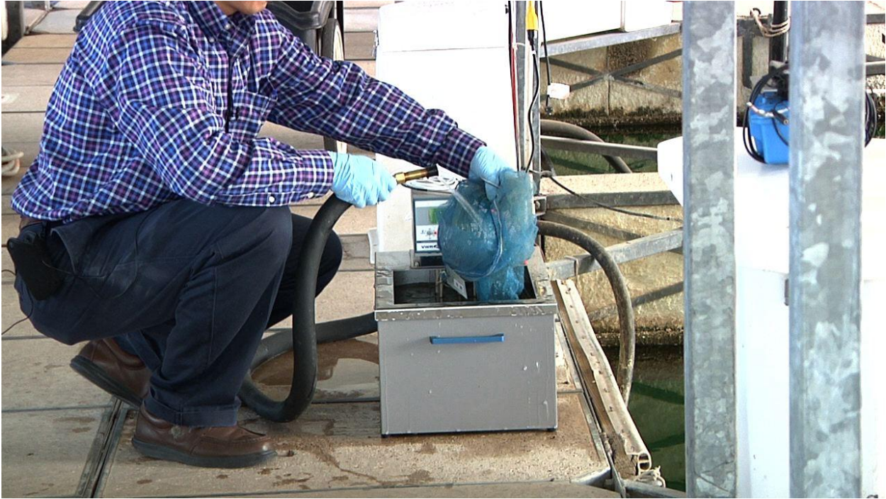
Dr. David Wong (UNLV) Testing Effect of Hot Water Spray on Live Quagga Mussels at Lake Mead
