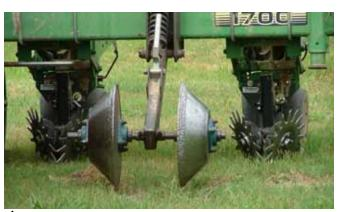
Figure 8-17. Example of planter attachments available to manage heavy residue from crops or cover crops in conservation tillage.
