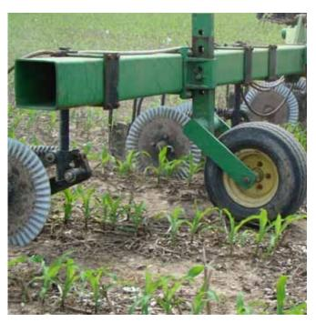
Figure 4-3. Side view of liquid fertilizer applicator in a conservation tillage system. The fluted coulter opens a narrow furrow in which liquid fertilizer is dropped behind the knife that follows the coulter.
