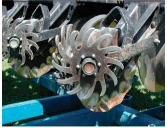
Figure 8–2. Residue cleaners with curved fingers
