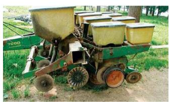
Figure 8-8. A planter mounted with a bubble coulter.
