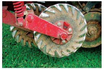
Figure 8–9. A fluted coulter with angled waves to facilitate soil penetration and reduce soil disturbance.
