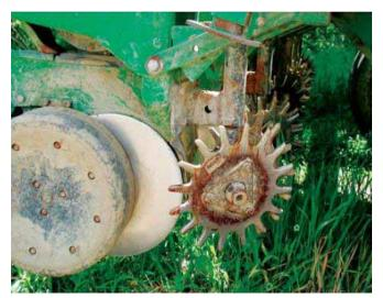
Figure 8-3. Residue cleaners with straight fingers.
