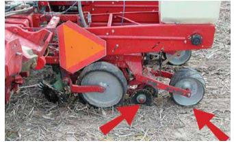
Figure 8-11. Case-IH rubber closing wheel.
