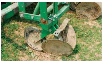
Figure 8-5. Residue cleaners with concave disks.
