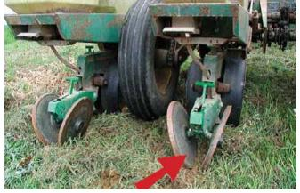
Figure 8-10. Cast-iron closing wheels.
