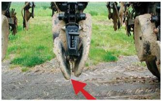
Figure 8-12. Rubber closing wheels.
