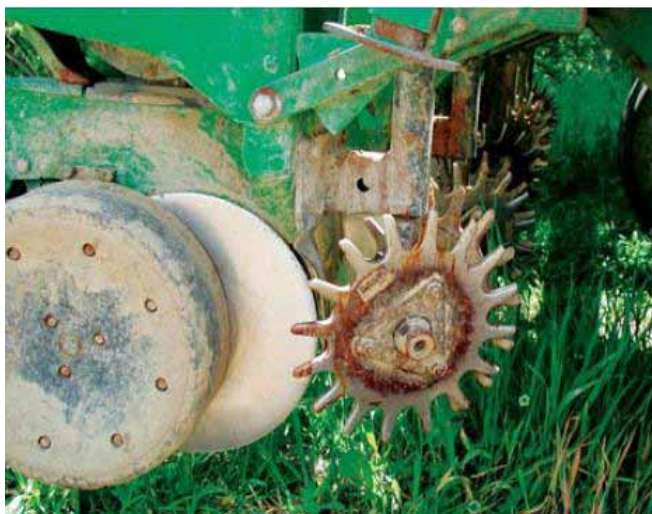
Figure 8-3. Residue cleaners with straight fingers.
