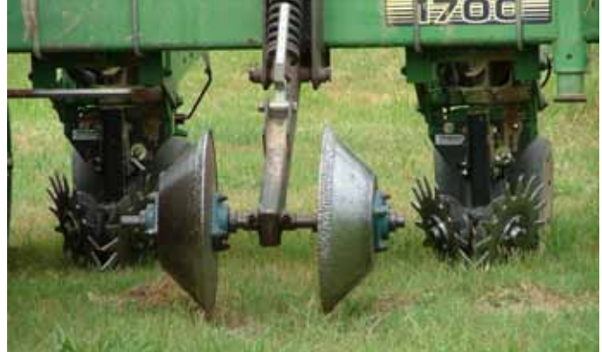
Figure 8-17. Example of planter attachments available to manage heavy residue from crops or cover crops in conservation tillage.
