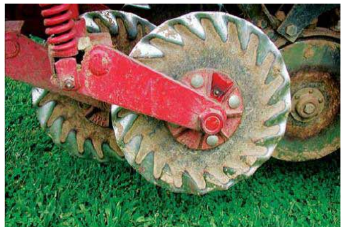
Figure 8-9. A fluted couler with angled waves to facilitate soil penetration and reduce soil disturbance.
