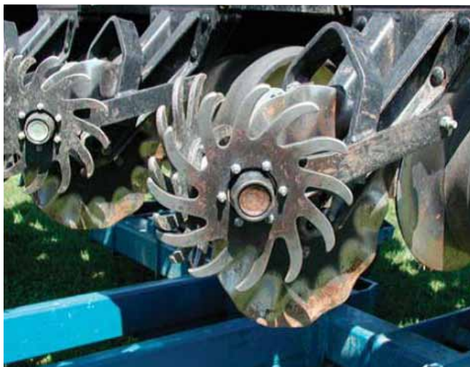
Figure 8-2. Residue cleaners with curved fingers
