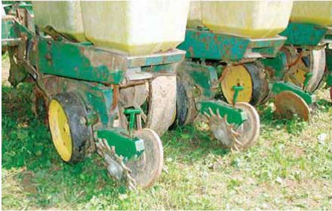
Figure 8-14. Some farmers mount one fingered and one cast iron closing wheel on a planter unit.
