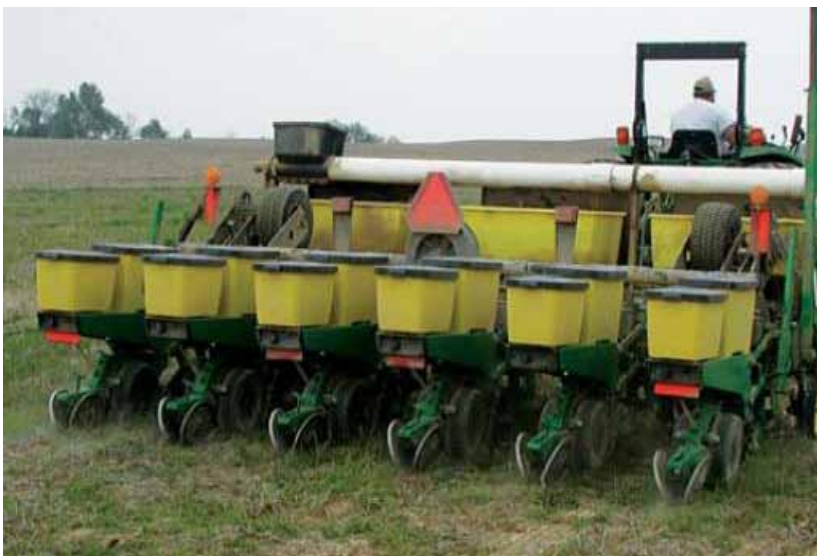
Figure 8-1. Six-row conservation tillage planter.
