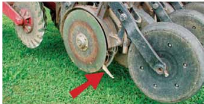
Figure 8-6. Seed firmer on a drill also pushes the seed into the bottom of the seed slot.
