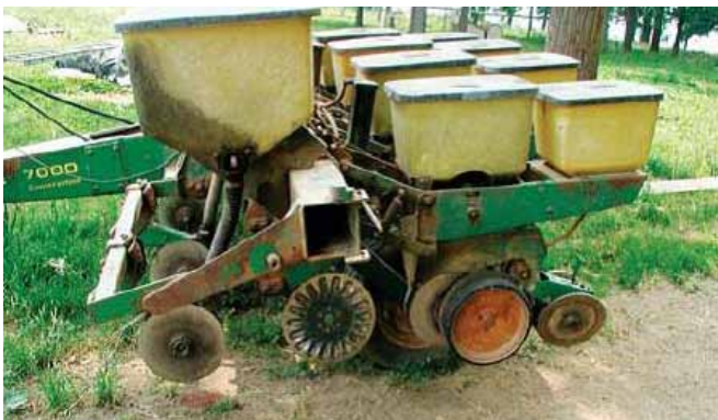
Figure 8-8. A planter mounted with a bubble couler.
