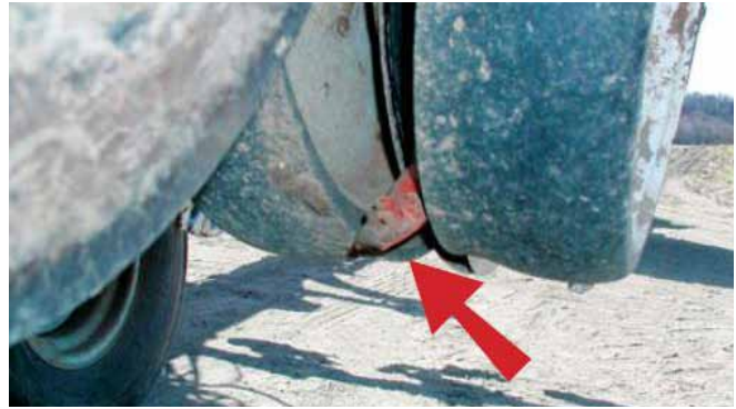
Figure 8-4. A seed firmer on a planter pushes the seed down into the seed slot to achieve optimum seed depth control. Pop-up fertilizer can be applied through the seed firmer.
