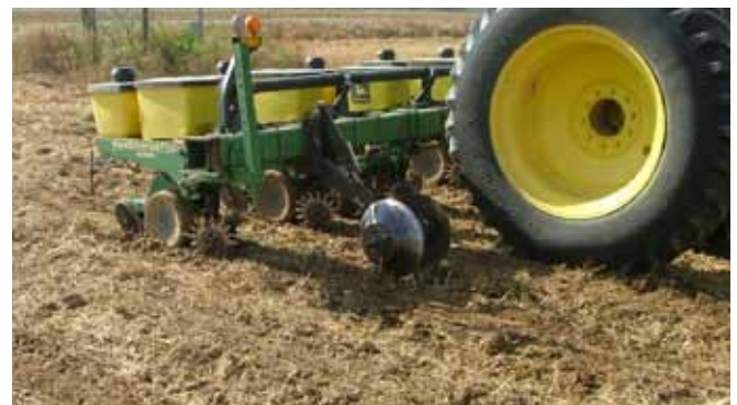
Figure 8-17. Example of planter attachments available to manage heavy residue from crops or cover crops in conservation tillage.
