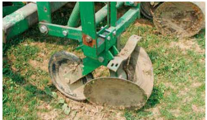
Figure 8-5. Residue cleaners with concave disks.
