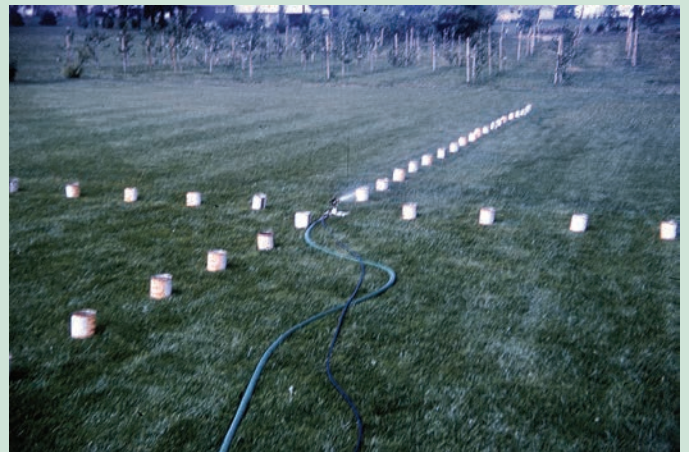
Checking Sprinkler Coverage
