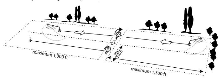
Figure 2. Layout of a hard-hose drag traveler. Travel lanes are 100-360 feet apart, depending on sprinkler capacity and diameter coverage.
