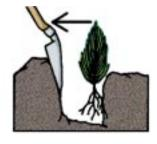
2. Straighten back of hole and insert tree at proper depth.
