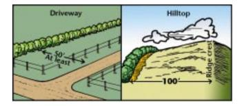
Figure 23. Living snow fences should be located back from driveways and roads. Place hilltop fences 100 feet on the windward side of ridge crests.
