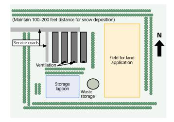
**Figure 10.** Hypothetical windbreak system design for a typical swine production facility. Courtesy lowa State University.
