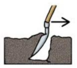
Insert shovel vertically with blade reversed, push handle forward, then pull soil back and out of hole.
