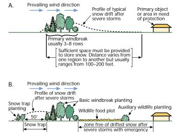
**Figure 19.** Locate windbreaks so the snow accumulation zone does not impact driveways and other structures.
