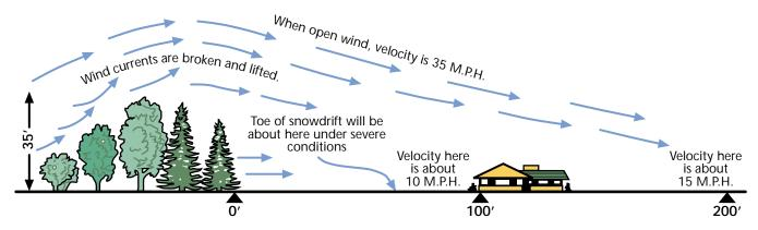
**Figure 1.** A dense windbreak that is properly designed and correctly located will reduce winds and control snow drifting. Note that a "traditional design" windbreak is illustrated here.
