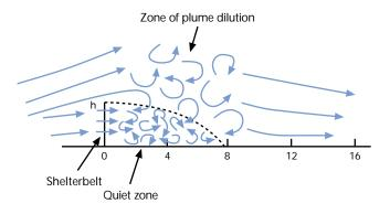
**Figure 11.** Schematic representation of turbulence and zone of potential odor dilution. Courtesy lowa State University.
