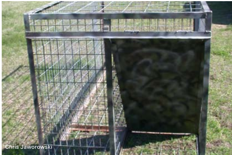
The portable cage trap can be easily moved from site to site, a vital capability for some managers. This particular trap is outfitted with a rooter door.
