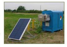
reaching 180 feet. Each unit, which cost about \$6,000, included a 65-watt PV panel and a vacuum/canister pump assembly. The recovery system fully operated off-grid and could be transferred from one well to another, as needed.
