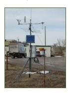
that guided removal actions along a five-mile stretch of contaminated soil. Information collected from both the weather stations and stream gauges was transmitted to an onsite trailer where it was recorded on a computer that operated data logging software. Use of this relatively inexpensive system avoided the need for frequent replacement of batteries or infeasible access to grid
