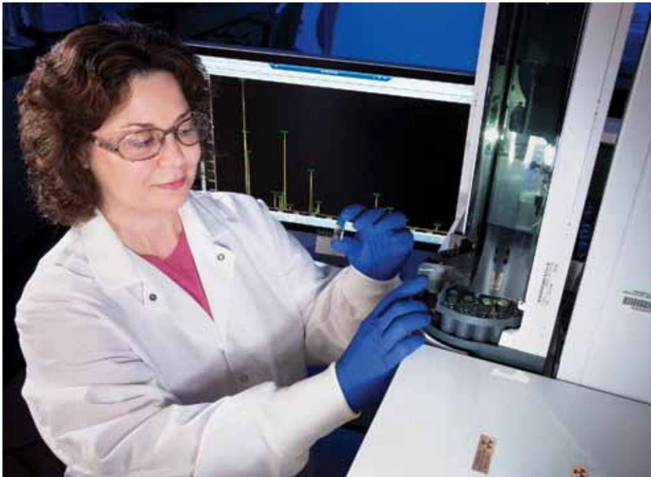
Using a gas chromatograph, technician Renee Russell analyzes the pesticide content of samples collected at various points along a vegetated drainage ditch. The goal is to determine how the ditches affect the fate and distribution of pesticides.
