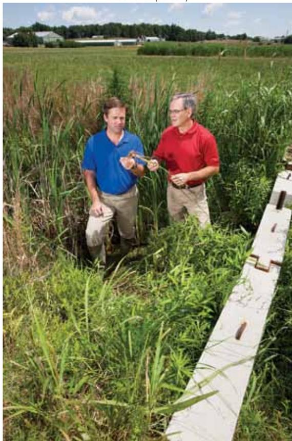
In tests to see how well vegetated drainage ditches like this one reduce agricultural pesticide and nutrient runoff, ecologist Matt Moore (left) and soil scientist Martin Locke assess the biomass of plants growing in the ditch.
