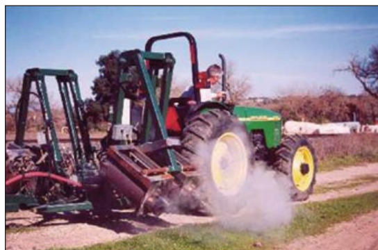
Weed control using steam by tractor. Photo by Dr. Thaddeus Gourd, Colorado State University Cooperative Extension for Adams County
