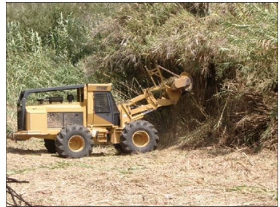
Hydroaxe machine cuts and mulches Arundo donax in lower Topanga Canyon.
