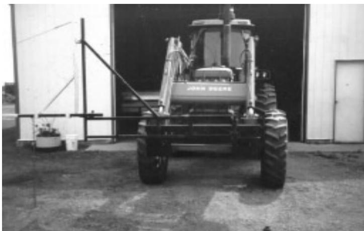
Flushing bars mounted on the front of mowing devices can reduce the number of birds killed when harvesting a field. The pictures here show how a flushing bar is connected to a self-propelled hay mower. To obtain specific information on how to build and mount a flushing bar on your tractor, please contact: Ducks Unlimited Canada / Alberta Prairie CARE office in Brooks at 403-362-4827 (<http://www.ducks.ca>). Photos courtesy Ducks Unlimited Canada.
