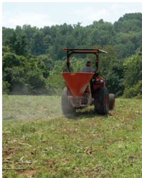
Fig. 3.13 Fertilizer applications are most easily accomplished with a cyclone spreader. Calibrating the spreader prior to fertilizer applications is just as important as calibrating it prior to sowing seed! Here, fertilizer is being spread prior to disking and planting a warm-season food plot.
