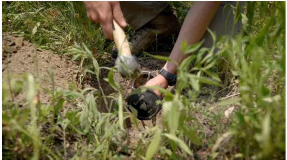
University of Missouri graduate student Will Rumpf gathering soil samples to measure bulk density. (USDA Forest Service photo by Preston Keres)
