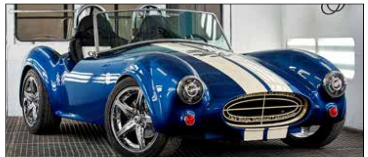
This Shelby Cobra was 3D printed at the Department of Energy's Manufacturing Demonstration Facility at the Oak Ridge National Laboratory.
