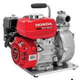
WH15XT2A HONDA 1-1/2" High Pressure Pump 57 psi max., 98 gal./min. capacity Weighs 49 lbs.
