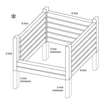
\*These are the dimensions for a single compost bin using 8 foot landscape timbers stacked on top of each other. Corner posts should be at least 3 feet below ground with 4 feet above ground. When building three bins side by side (as in the diagram above), you will need a total of 8 posts to create three separate bins.
