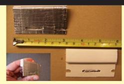
Cut strips into 3-inch pieces using miter saw (tin snips work for small projects). To reduce splintering, use a fine-toothed plywood blade (200 teeth), vinyl siding blade, or tile saw blade (*Caution: Always follow manufacture's guidelines for safety when operating power tools*). Multiple undersill strips can be stacked and cut at once to expedite production. Cut slowly.
