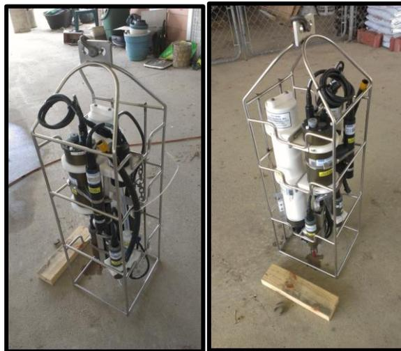
**Figure 13** . Photos of the USM CTD package with sensors.
