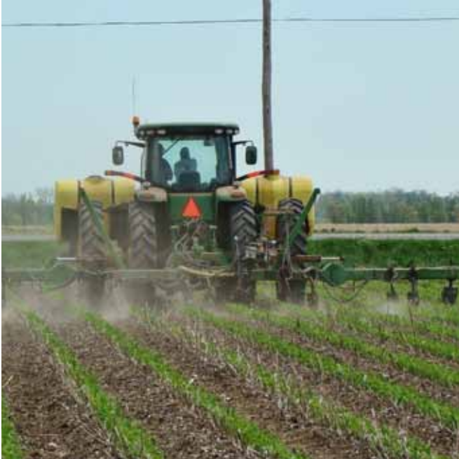
Figure 4-2. Fertilizer sidedress application of nitrogen in a conservation tillage system. Note the fertilizer is knifed in several inches away from the crop row to prevent losses due to volatilization and reduce the risk of fertilizer injury.
