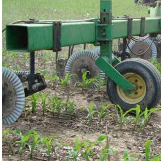
Figure 4-3. Side view of liquid fertilizer applicator in a conservation tillage system. The fluted coulters opens a narrow furrow in which liquid fertilizer is dropped behind the knife that follows the coulters.
