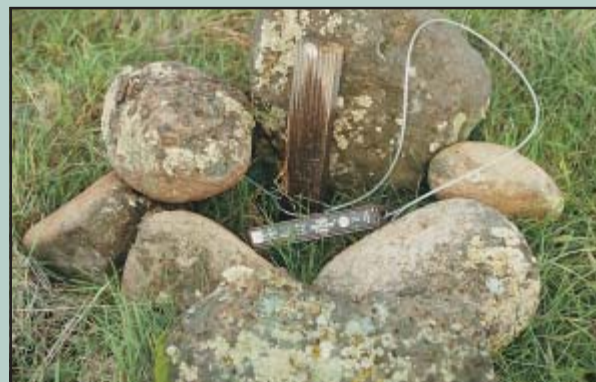
Air temperature logger placement.
